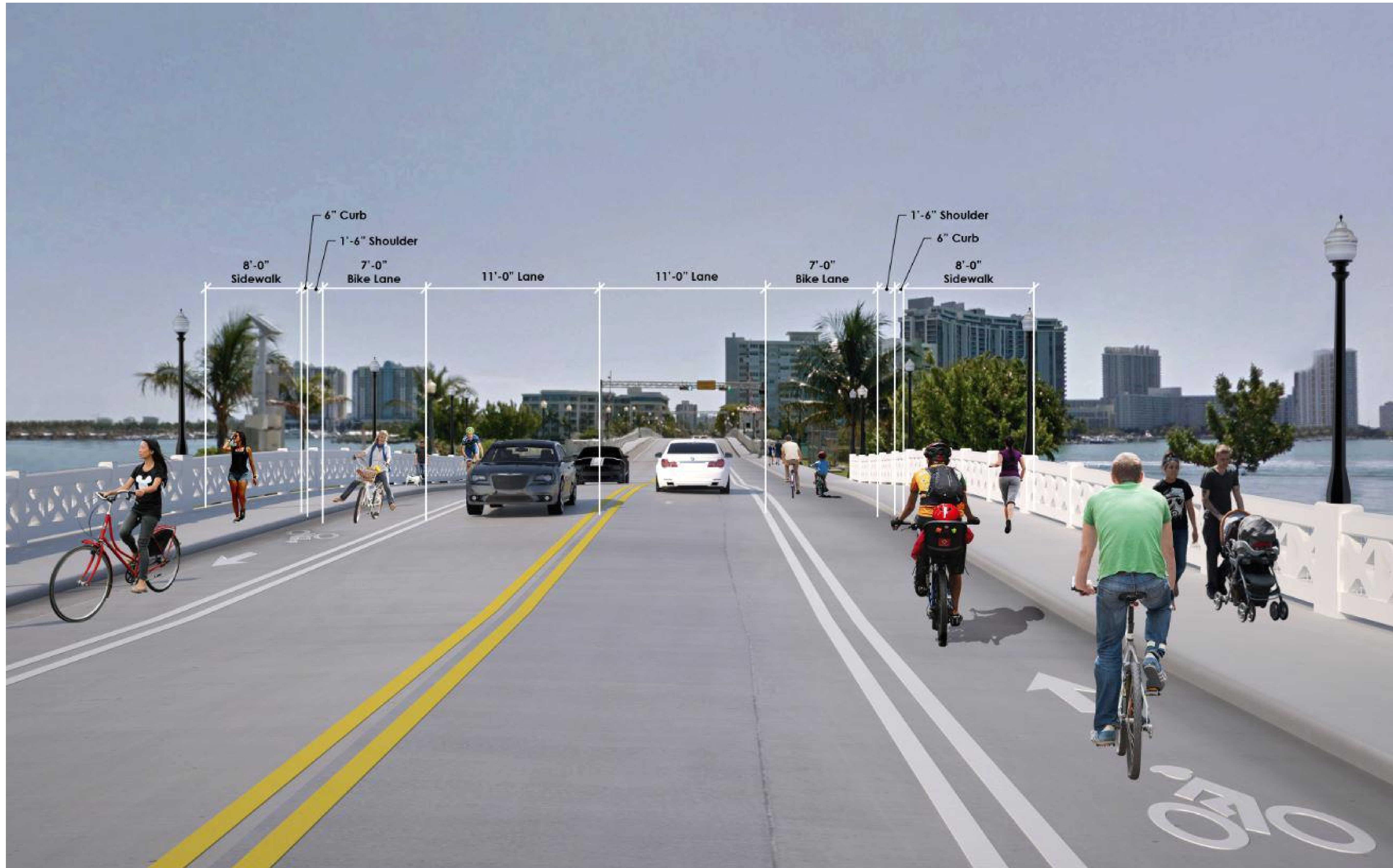
FIXED BRIDGE TYPICAL SECTION
