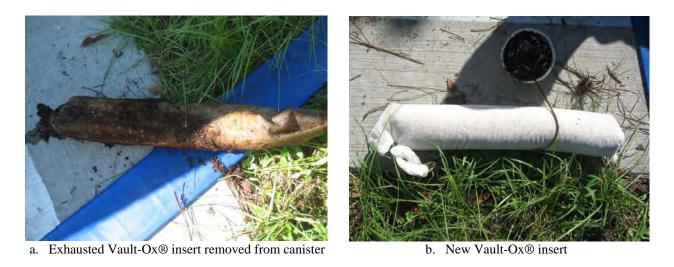
Figure 3-11. Photographs of Exhausted and New Vault-Ox® Inserts.
