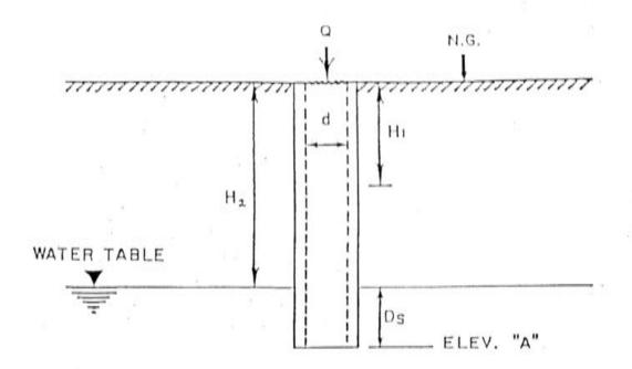
$$K = \frac{4Q}{\pi d(2H_2^2 + 4H_2D_S + H_2d)}$$
