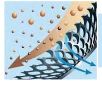
Continuous deflective separation — water velocities within the swirl chamber continually shear debris off the screen to keep it clean
