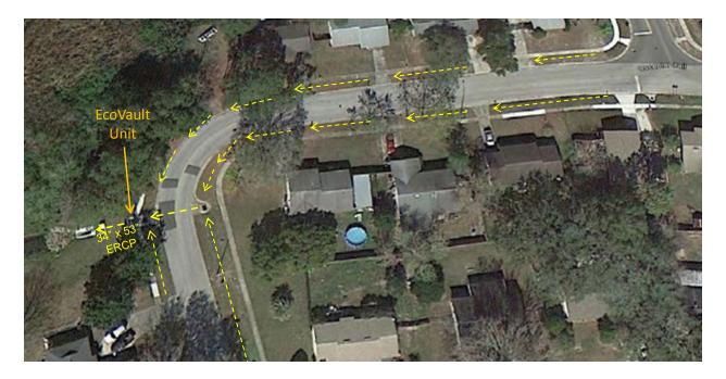
Figure 2-8. Drainage Patterns in the Vicinity of the Lake Hodge Baffle Box Site.
