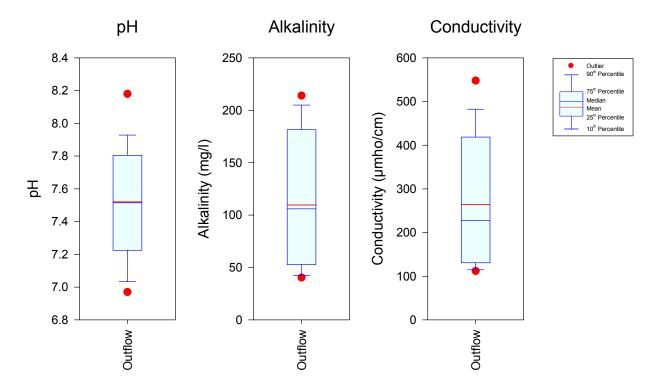
Figure 4-44. Statistical Summary of Outflow Concentrations of pH, Alkalinity, and Conductivity at the Lake Concord Suntree Baffle Box Site.
