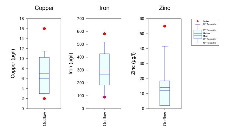
Figure 4-51. Statistical Summary of Outflow Concentrations of Copper, Iron, and Zinc at the Lake Concord Suntree Baffle Box Site.
