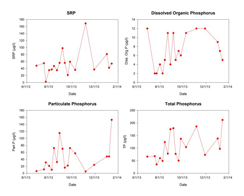
Figure 4-48. Characteristics of Outflow Concentrations of Phosphorus Species at the Lake Concord Suntree Baffle Box Site.
