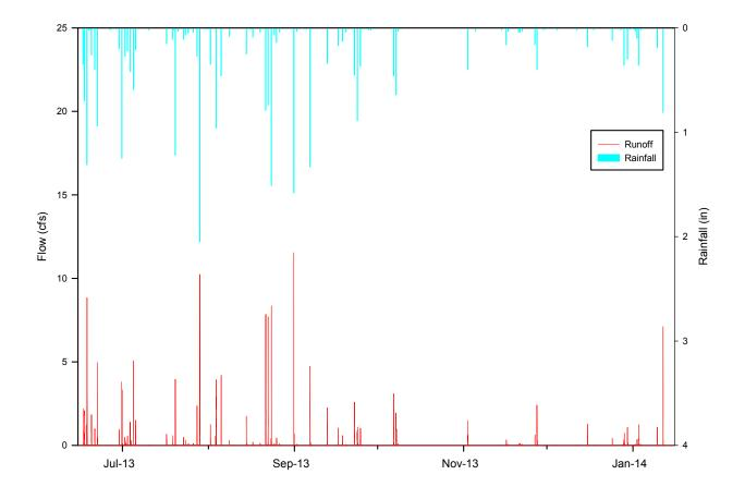
Figure 4-4. Measured Runoff Hydrographs at the San Pablo EcoVault® Site from June 15, 2013-January 15, 2014.
