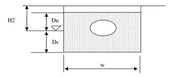
\*Provided Water Quality Treatment is calculated based upon the formulas presented in Appendix F from the SFWMD Permit Information Manual Volume IV for French Drains, where the saturated depth of trench is greater than the non-saturated depth of trench.
