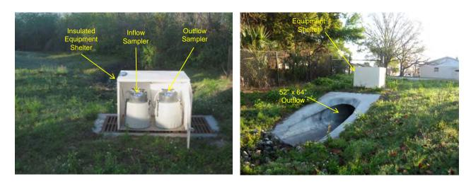
Figure 3-2. Overview of Sampling Equipment Installed at the Lake Hodge Site.
