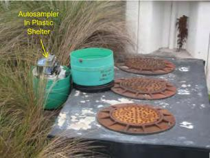
Figure 3-8. Photographs of Sampling Equipment Used at the Lake Concord Suntree Baffle Box Site.
