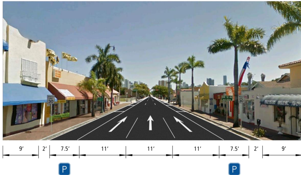
Figure 1-3: Existing Roadway Typical Section of Eastbound SR 90
