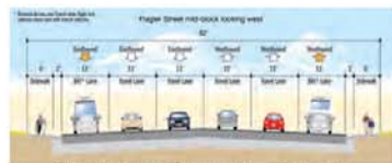
Alternative 5. BRT - Concurrent Flow, Shared Right Side (BAT); Repurposed Lanes
