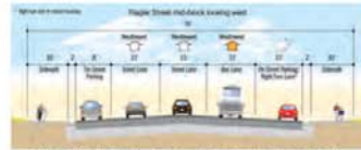
Alternative 6. BRT - Concurrent Flow, Exclusive Right Side Offset; Repurposed Lanes
