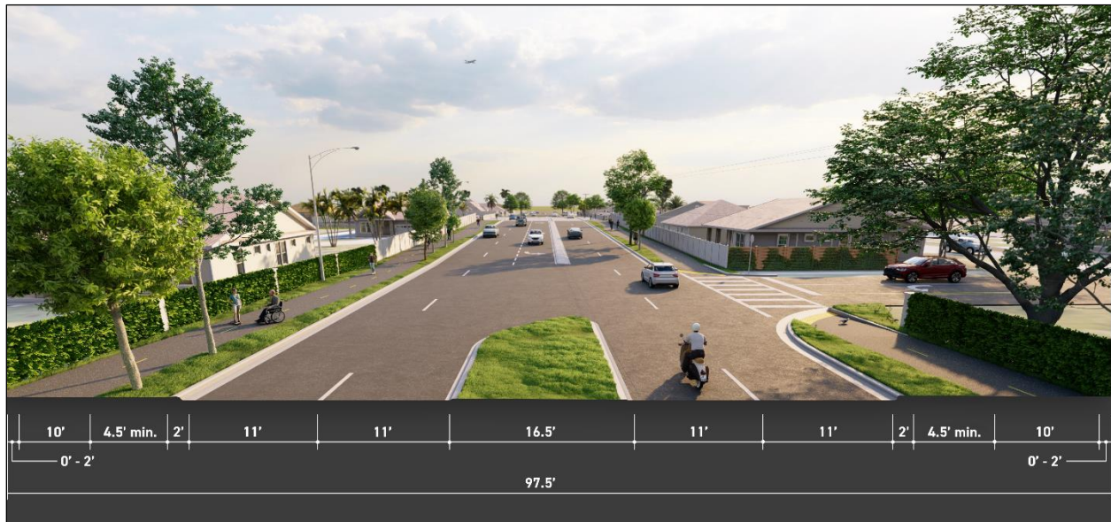
Figure 2-7: Build Alternative 2 Typical Section
