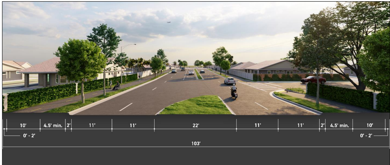
Figure 2-12: Build Alternative 3 Typical Section
