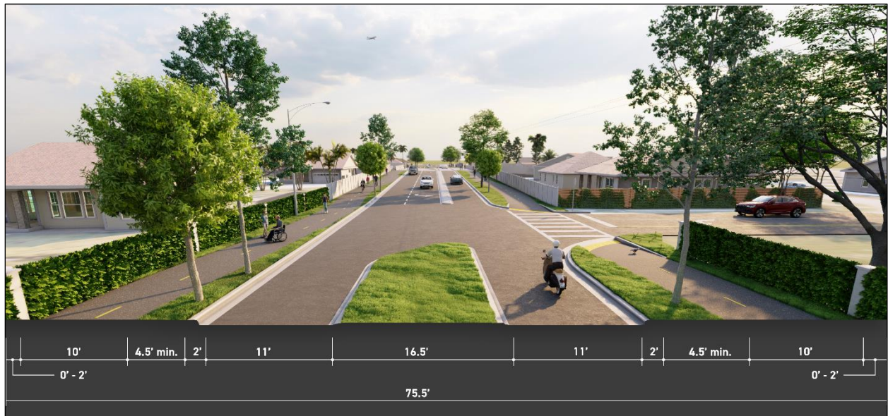
Figure 2-3: Build Alternative 1 Typical Section
