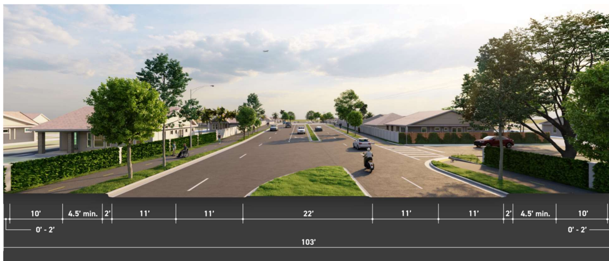
Figure 4-3 Build Alternative 3 Typical Section
