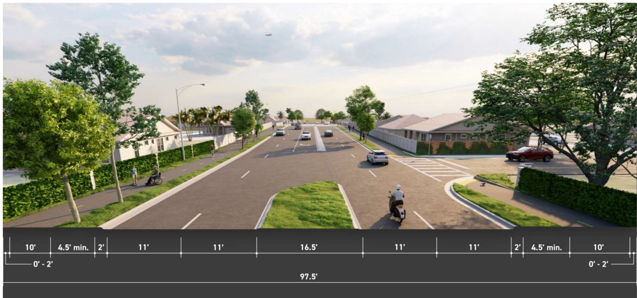
Figure 4-2: Build Alternative 2 Typical Section
