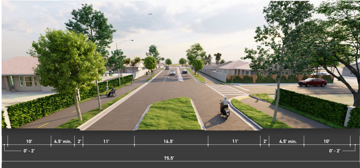
Figure 4-1: Build Alternative 1 Typical Section
