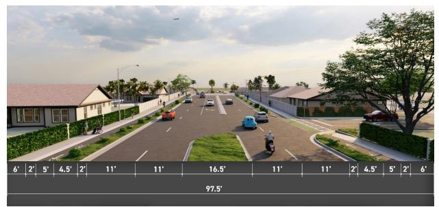
Figure 1-4 Build Alternative 2 Typical Section
