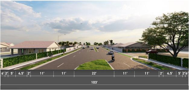
Figure 4-14 Build Alternative 3 Typical Section
