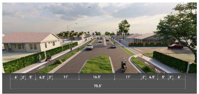
Figure 4-12 Build Alternative 1 Typical Section
