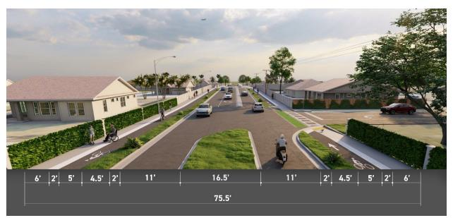
Figure 1-3 Build Alternative 1 Typical Section
