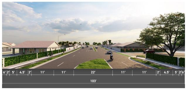
Figure 1-5 Build Alternative 3 Typical Section
