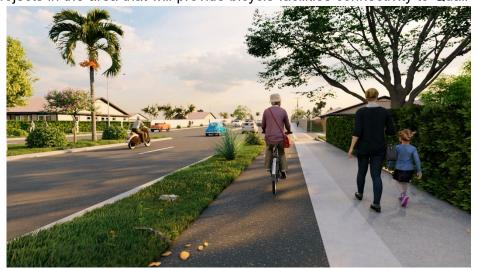
Figure 6-3 Sidewalk Level Separated Bicycle Lane
