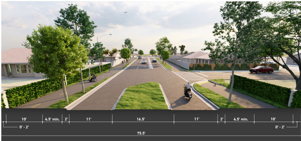
Figure 1-4: Build Alternative 1 Typical Section
