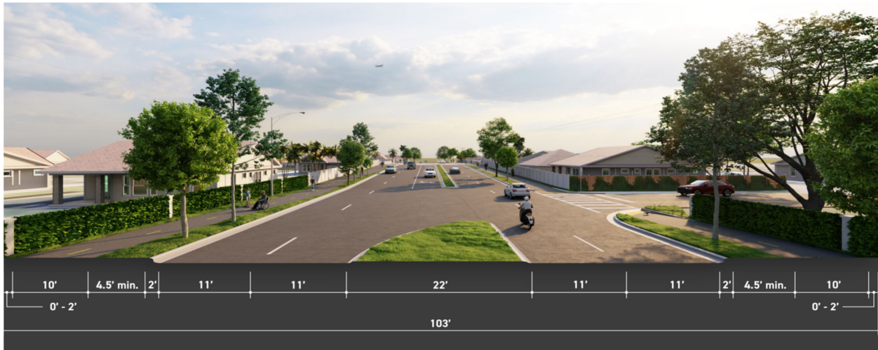
Figure 1-5: Build Alternative 3 Typical Section
