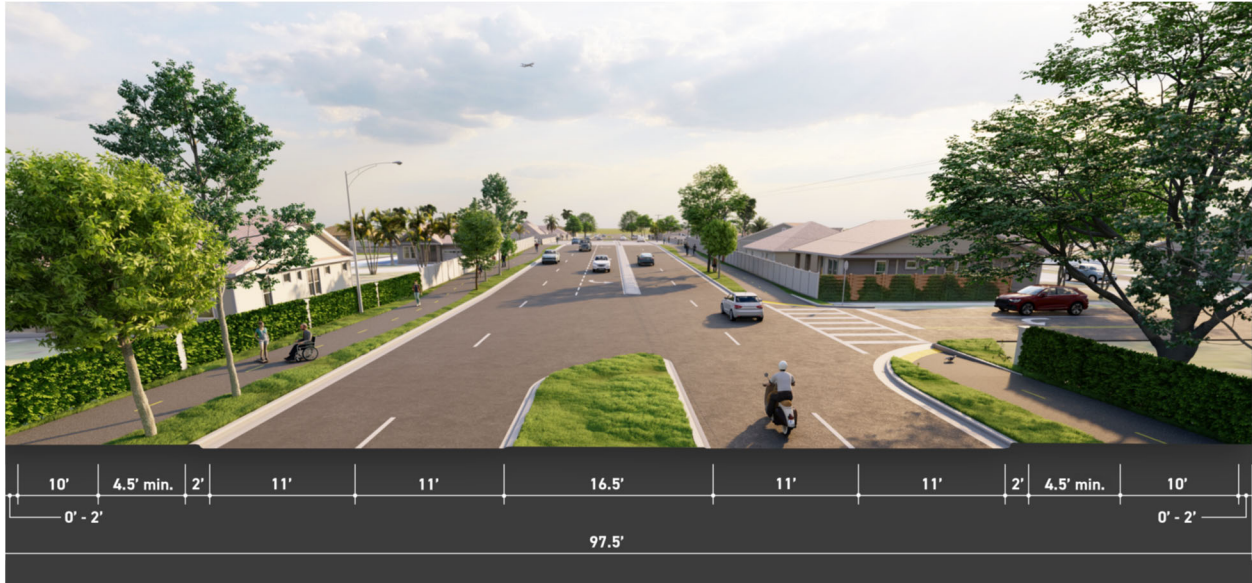
Figure 1-6: Build Alternative 2 Typical Section
