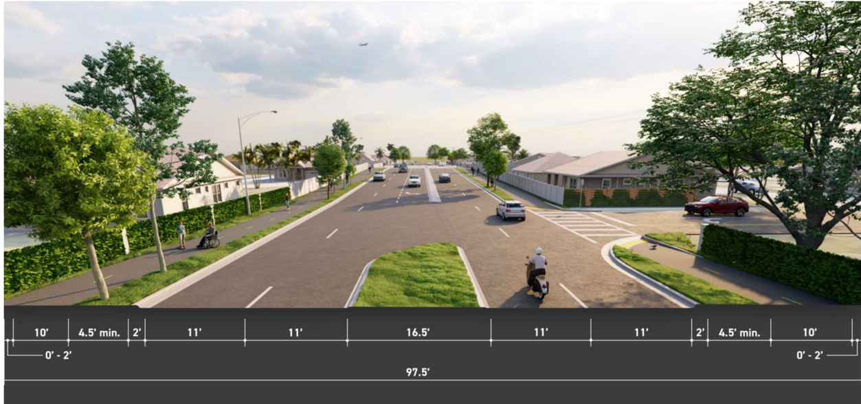
Figure 4-2: Build Alternative 2 Typical Section
