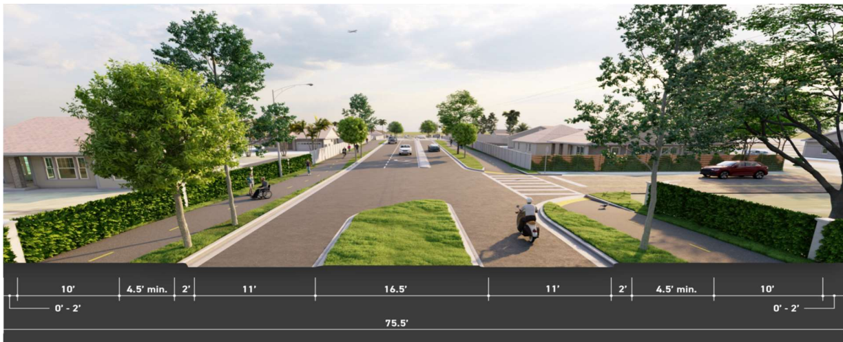
Figure 4-1: Build Alternative 1 Typical Section
