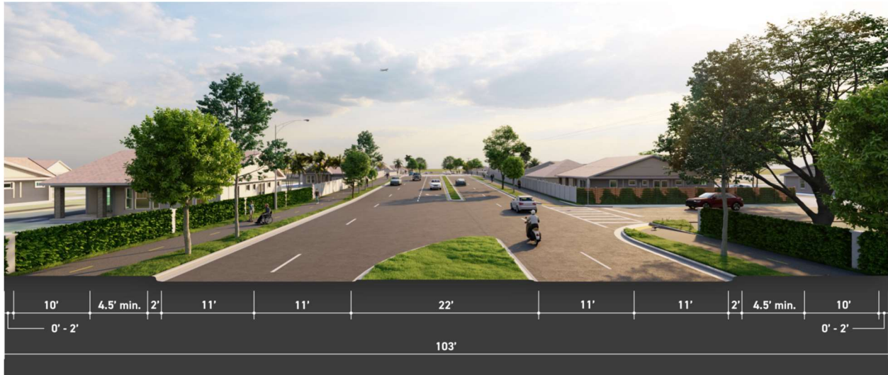
Figure 4-3: Build Alternative 3 Typical Section
